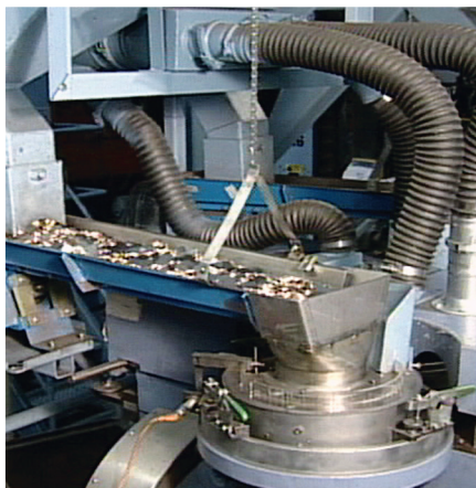
The upsetting mill forms a rim on each blank coin.
