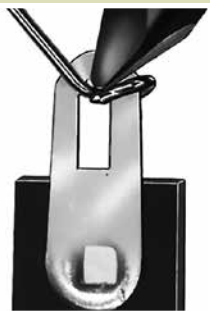
Heat the wire and the lug.
