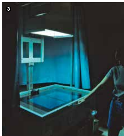
3 Expose the plate to light.
