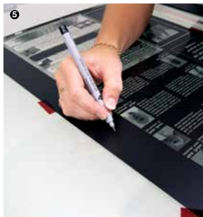
Cover any nonimage marks with opaque.
