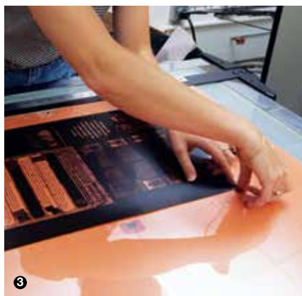
Tape the negative to the goldenrod paper.
