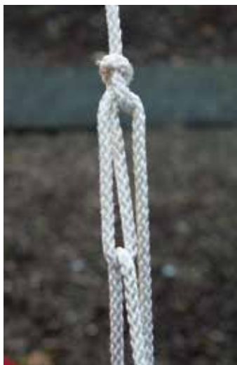
The trucker's hitch does not slip when tied properly.
