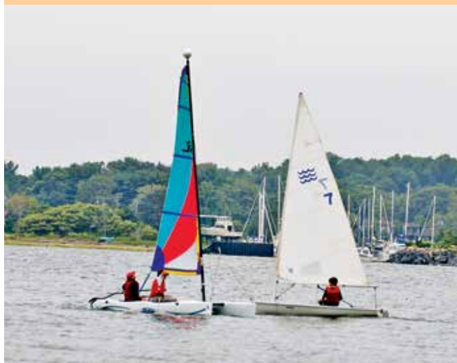
The boat on the left is on starboard tack. The boat on the right is on port tack.
