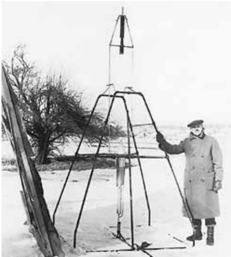
Dr. Robert H. Goddard standing next to the rocket that would make the world’s first liquid propellant rocket flight on March 16, 1926.
