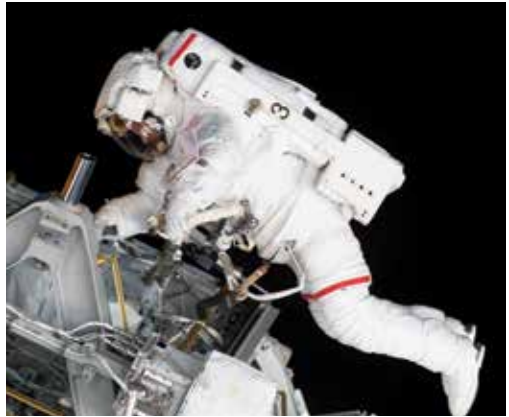
Crew members wear small gas jetpacks that can get them back to the station if they get separated from the spacecraft.
