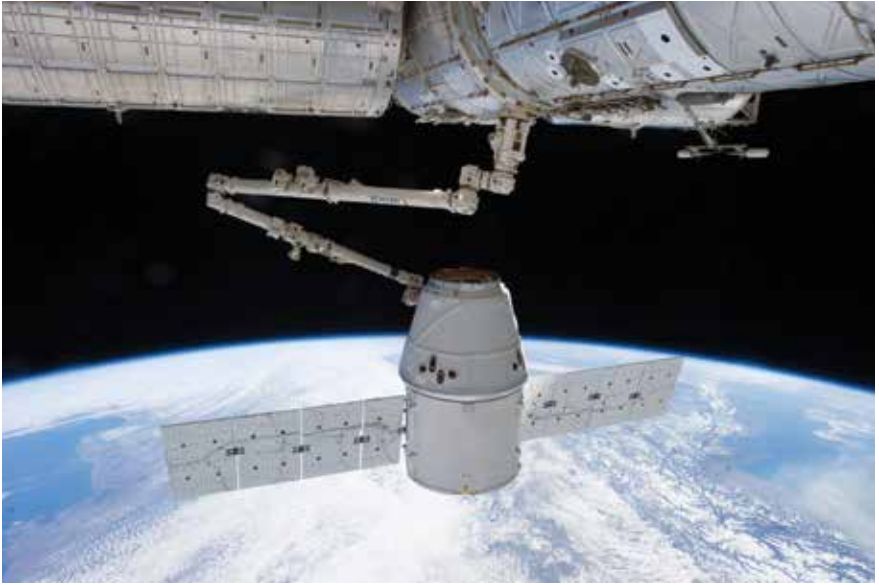
The ISS's robot arm captures the SpaceX Dragon spacecraft as it approaches on a resupply mission.
