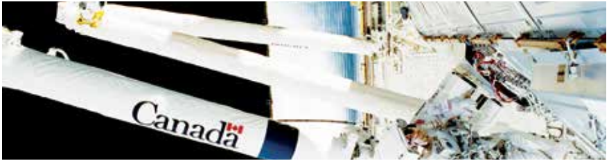
Canada's Space Station Remote Manipulator System can creep slowly along the outside of the space station like an inchworm.
