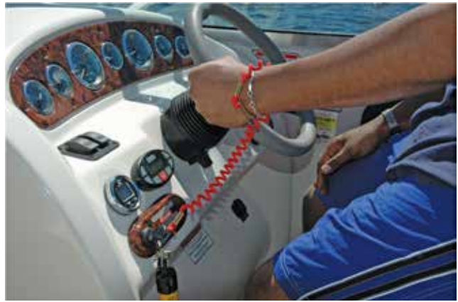
Attach the safety lanyard and run the blower prior to starting the engine.
