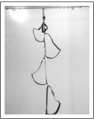
A 3:1 jigger pulley system can be used to raise a participant. A jigger system is compact and can be prerigged into a rescue pack. The jigger system will be attached to an upper anchor by the staff, and the lower end of the jigger system will be lowered to the participant who will connect it to his or her harness. The participant can be raised by a haul team on the ground, or if the participant needs to be raised only a few feet the staff on the event may be able to do the raising.
