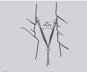
The forces on the individual points of the anchor system increase as the angle between the anchor points increases.
