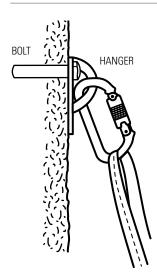
While chocks and camming devices are removed at the end of a climbing session, bolts are secured in holes drilled into the rock and are permanent. Likewise, the bolt hanger (a bent strip of metal secured by a nut or bolt) also stays in place, providing the means to use a carabiner to connect to the anchoring system.
