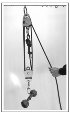
Applications of a 5:1 system are similar to the uses for a 3:1 but when more mechanical advantage might be needed due to the distance the load needs to be raised. Another reason to need more mechanical advantage might be because there aren't enough people around for the haul team.
