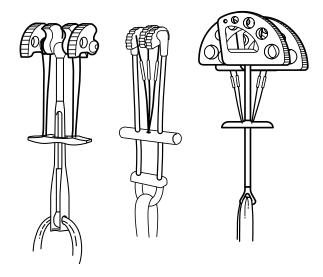
A spring-loaded camming device (SLCD) placed in a crack of a width for which it was designed can provide a very solid anchor point. The cams of the device should not be too open or too closed when they are released inside the crack. Proper placement allows for maximum grip while still being easy to extract. Orient the stem of an SLCD in line with the pull of any potential falls.
