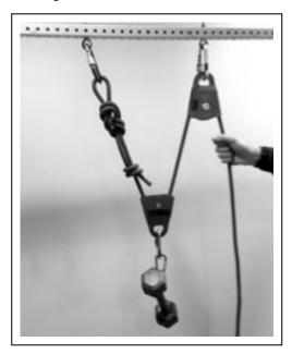
A 3:1 system could be used to hoist a participant on a natural site, to raise a person out of a cave, to raise a special needs participant to an element, to raise a person back up onto an element, or to lift a staff member or rescuer to assist a participant. A top-roped belay line can be converted to a 3:1 to lift a climber.
