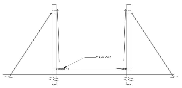
**NOTE:** TURNBUCKLES CAN BE USED FOR DISABLING EVENTS AS WELL AS TO MAINTAIN PROPER TENSION.
