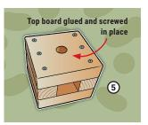
5. Glue and screw the top board onto the sides and base. Sand the slide until it moves smoothly in the square hole in the center of the dispenser.
