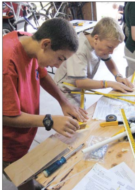
Scouts Quentin Marchetti, KDØKGJ (left) and Austin Armstrong, KDØKJP, prepare antenna segments for soldering during the tape-measure Yagi workshop.
