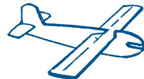
ASSEMBLE PARTS AND FASTEN PAPER CLIP (OR BOBBY PINS) TO NOSE. THE CURVE IN THE WING CREATES AN "AIR FOIL" TO HELP THIS TOY PLANE FLY IN THE SAME MANNER AS REAL PLANES.
