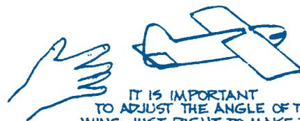
IT IS IMPORTANT TO ADJUST THE ANGLE OF THE WING JUST RIGHT TO MAKE THE PLANE FLY STRAIGHT. TRY TILTING IT A LITTLE AND WATCH THE PLANE LOOP-THE-LOOP OR NOSE-DIVE!
