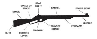
Spring-piston air guns use a manually operated lever, pivoting barrel, or other device to move a piston that in turn compresses a mainspring located in the frame or receiver portion of the gun.
