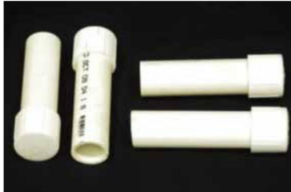
3. Place the four capped pieces inside the four perpendicular openings of the PVC furniture fitting.
