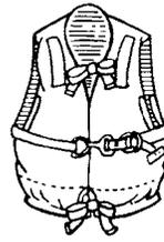
**Type I**—an approved device designed to turn an unconscious person in the water from a facedown position to a vertical or slightly backward position and to have more than 20 pounds of buoyancy. The device will maintain a vertical or slightly backward position and therefore greatly increase chances
